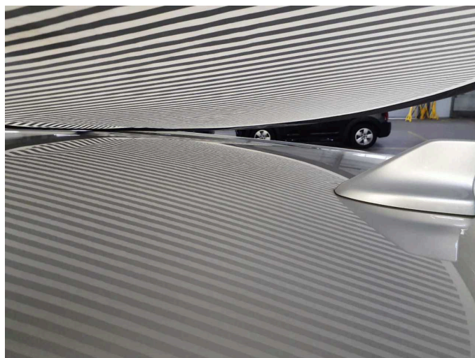
Damage 3: Body: Body - Damage by hail - Smooth repair work
