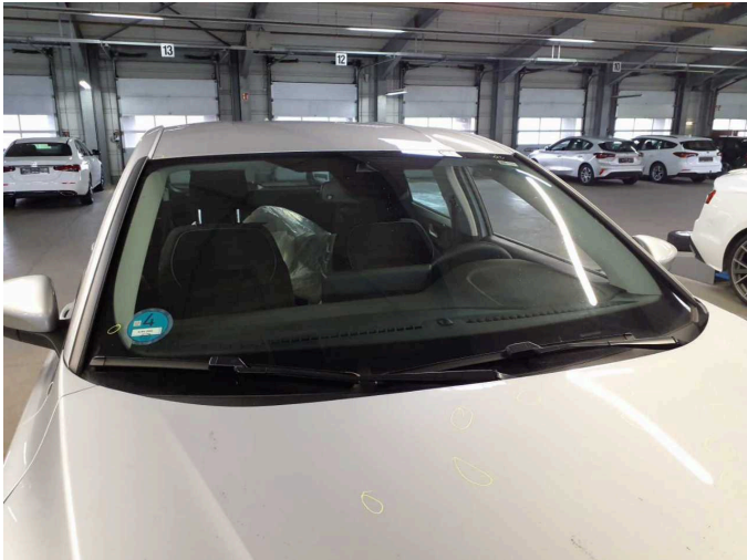
Damage 2: Vehicle glazing: Windscreen with lane departure assistant - Stone chips - Replace
