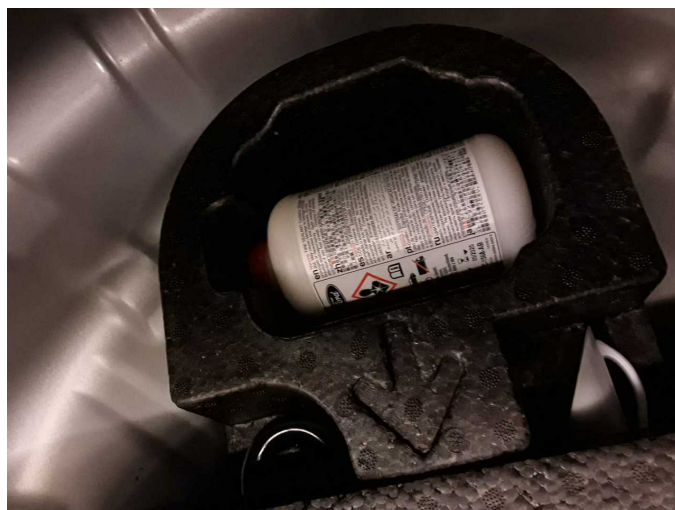
Damage 1: Equipment: Tirefit filler - Expired - Replace
