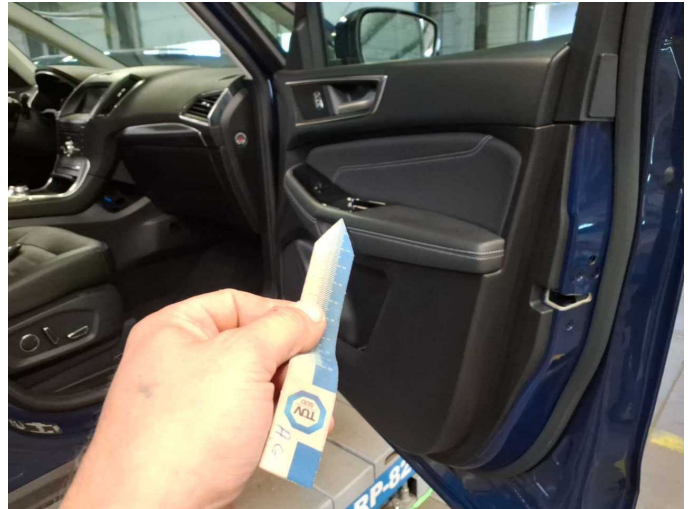
Damage 9: Trim / covers: Door trim - front right side - Broken / torn - Replace
