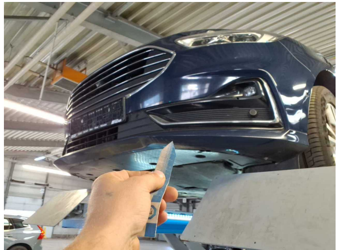
Damage 10: Front bumper: Spoiler - Scratched - Paint
