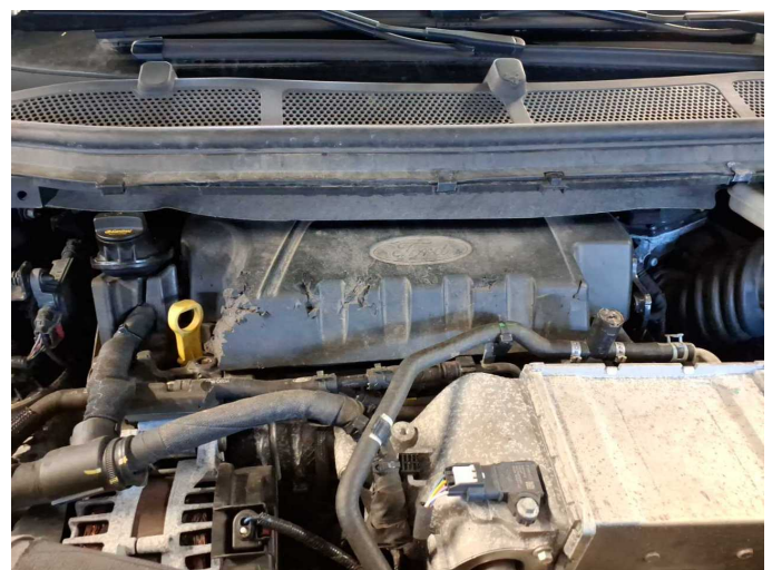
Damage 6: Engine: Engine cover - top / cover (Marderschaden) - Broken / torn - Replace
