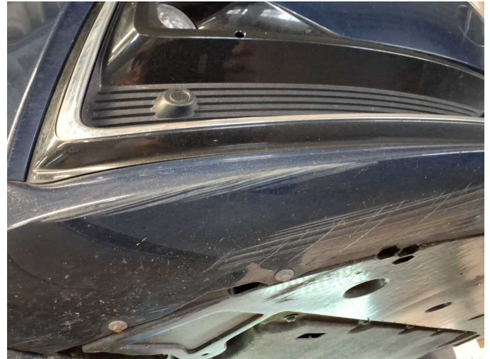
Damage 10: Front bumper: Spoiler - Scratched - Paint
