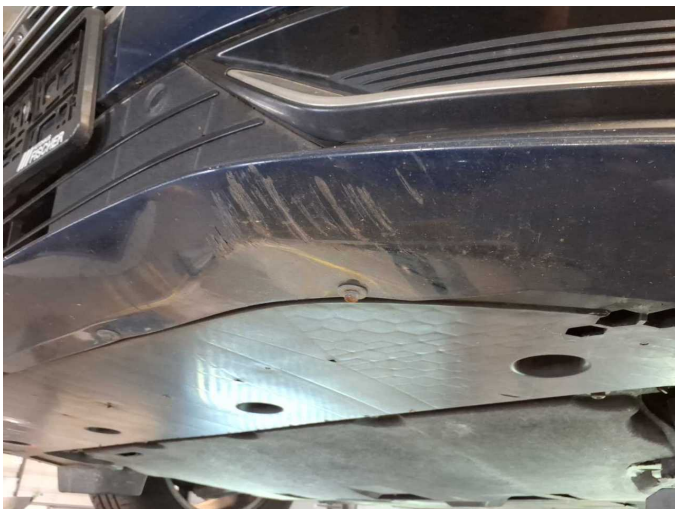
Damage 10: Front bumper: Spoiler - Scratched - Paint
