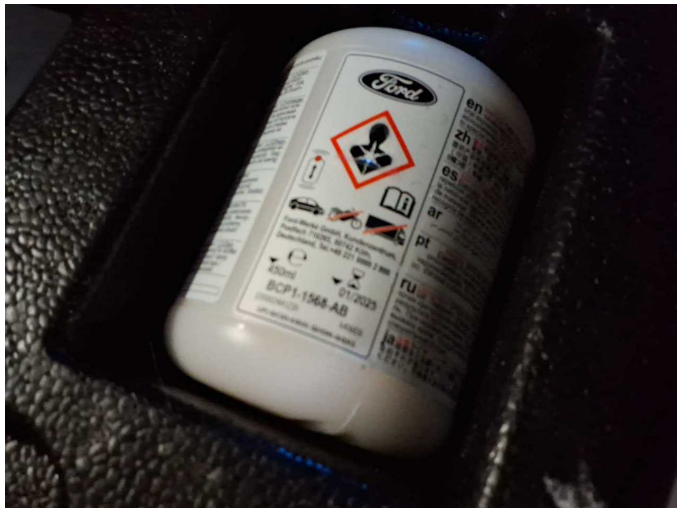
Damage 3: Equipment: Tirefit filler - Expired - Replace
