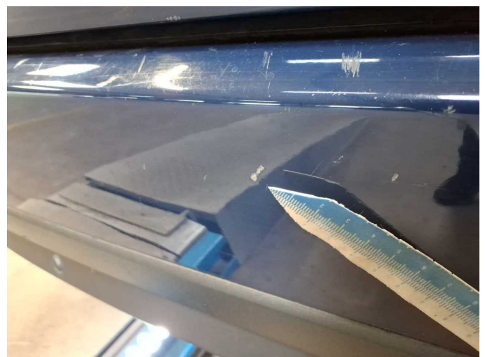
Damage 11: Rear bumper: Rear bumper - Scratch(es) - Paint
