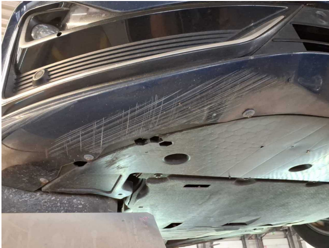
Damage 10: Front bumper: Spoiler - Scratched - Paint
