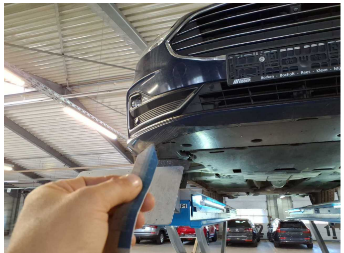
Damage 10: Front bumper: Spoiler - Scratched - Paint
