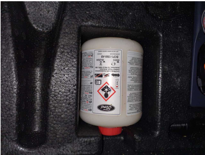
Damage 1: Equipment: Tirefit filler - Expired - Replace
