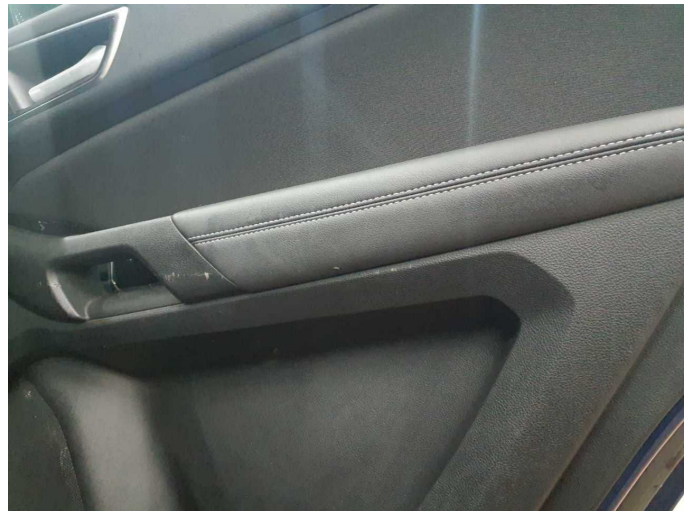
Damage 2: Trim / covers: Door trim - rear right side - Scratched - Loss in value
