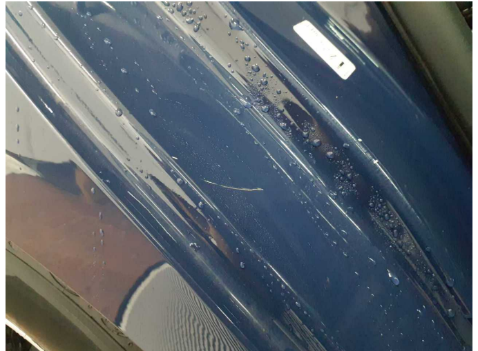
Damage 8: Side panel - rear right side: Sill - Scratched - Smart repair
