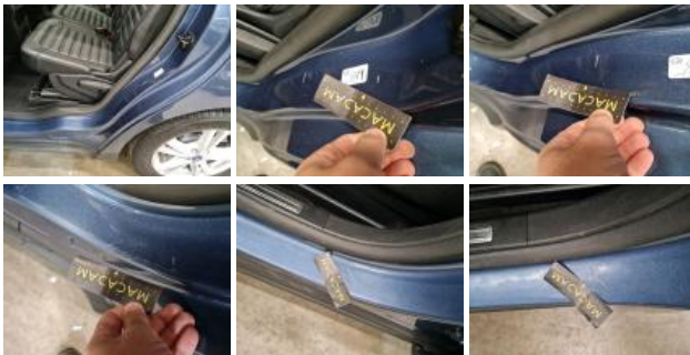
Porte ARG, Griffe(s), Acceptable
