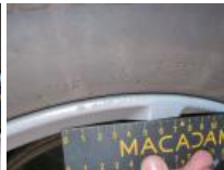
Wing FR, Scratch(es), Repair and paint (complete)
