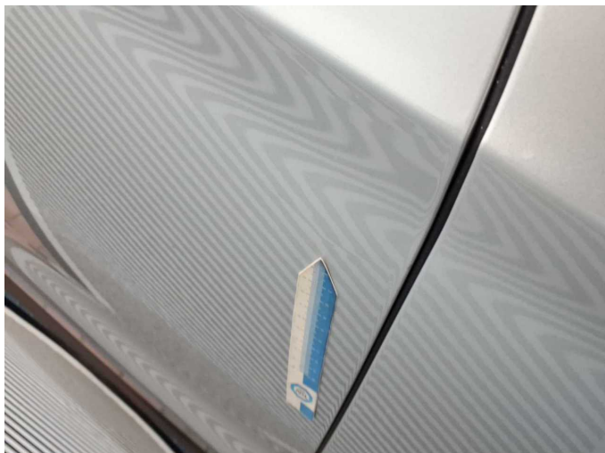
Damage 7: Door - rear right side: Door (Farbunterschied + Lackverlauf) - Unprofessionally repaired - Paint
