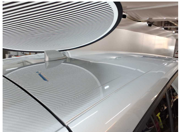
Damage 2: Roof: Roof - dent(s) - Smart repair
