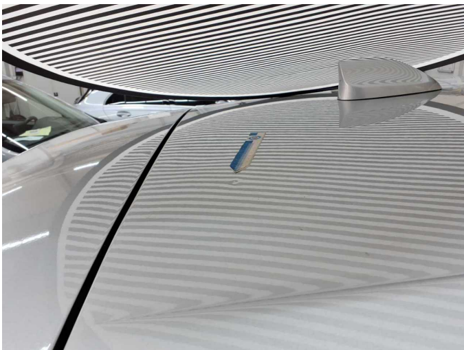
Damage 2: Roof: Roof - dent(s) - Smart repair
