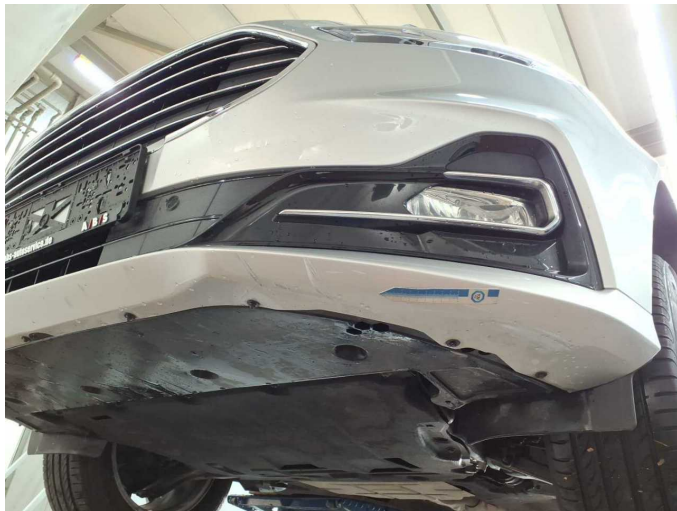
Damage 4: Front bumper: Spoiler - Scratched - Paint
