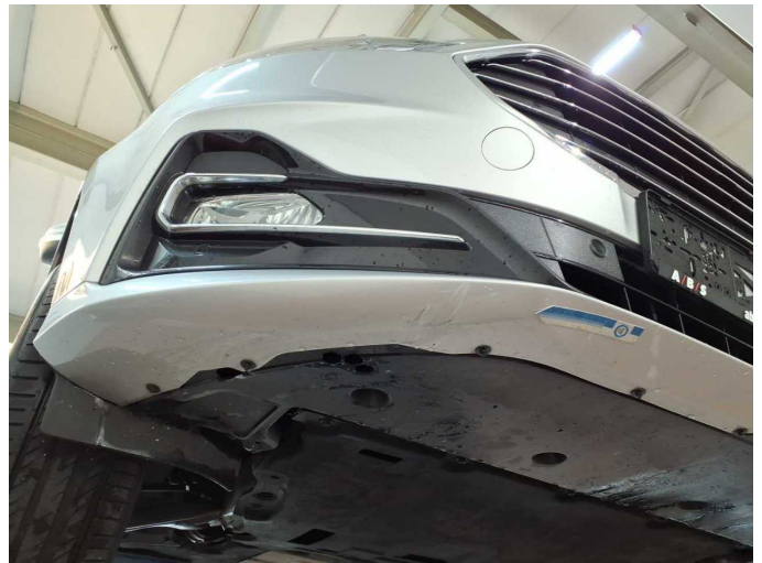
Damage 4: Front bumper: Spoiler - Scratched - Paint
