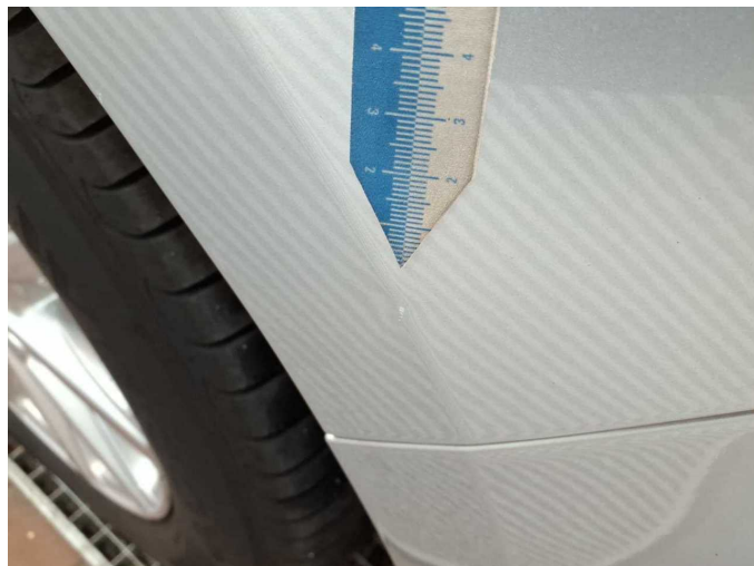
Damage 5: Mudguard - right side: Mudguard - right side - Dent / paintcoat damage - Paint
