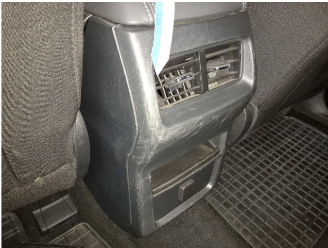
Damage 1: Instrument panel: Centre console - rear - Scratch(es) - Loss in value
