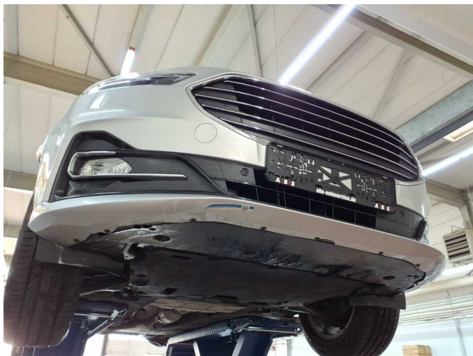
Damage 4: Front bumper: Spoiler - Scratched - Paint
