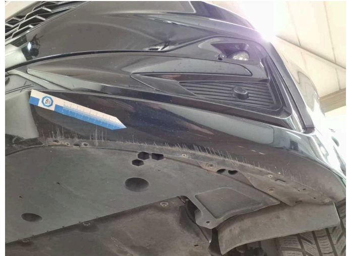
Damage 4: Front bumper: Spoiler - Scratched - Paint
