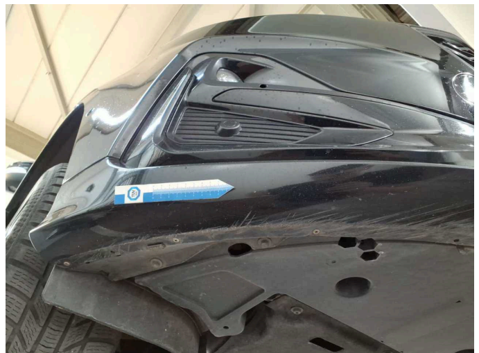
Damage 4: Front bumper: Spoiler - Scratched - Paint
