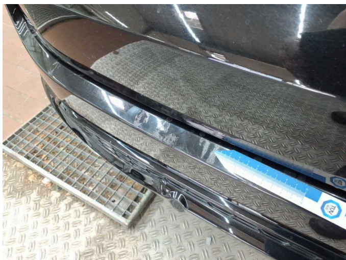
Damage 6: Rear bumper: Rear bumper - Scratch(es) - Paint
