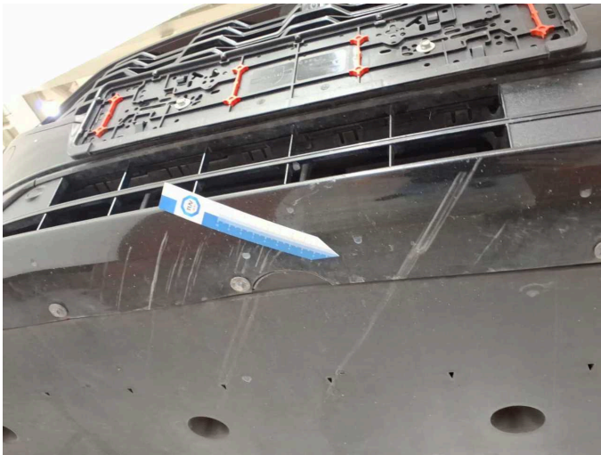
Damage 4: Front bumper: Spoiler - Scratched - Paint
