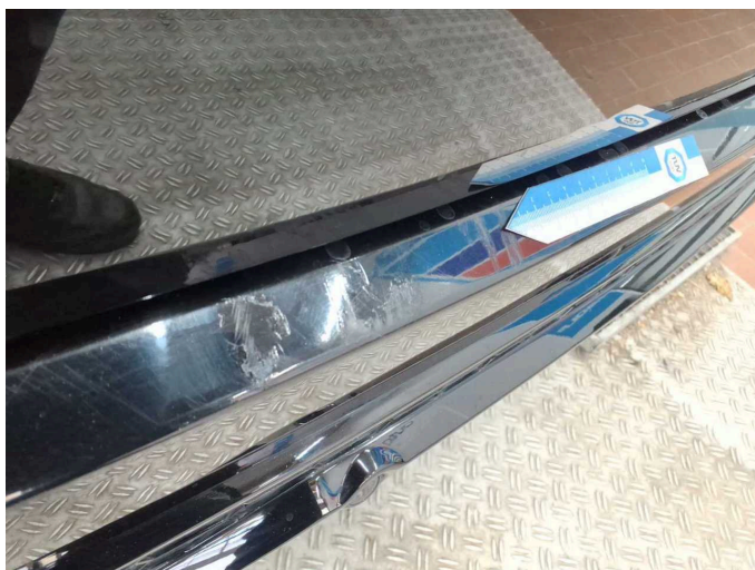
Damage 6: Rear bumper: Rear bumper - Scratch(es) - Paint
