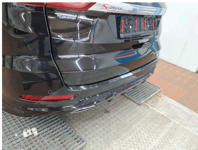
Damage 6: Rear bumper: Rear bumper - Scratch(es) - Paint
