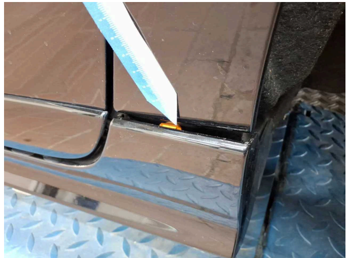
Damage 3: Sill - left side: Sill - Loose - Un- / install
