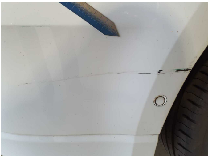
Damage 4: Rear bumper: Rear bumper - Scratch(es) - Paint
