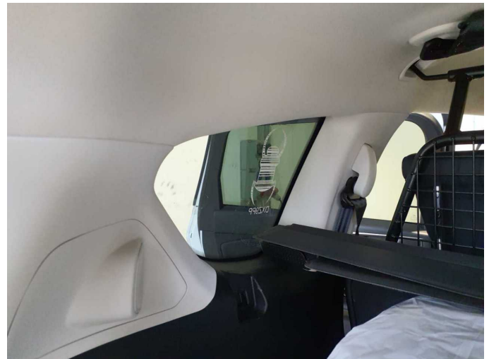
Damage 2: Vehicle glazing: Side window - rear left side - Glued / labelled - De-glue / neutralise
