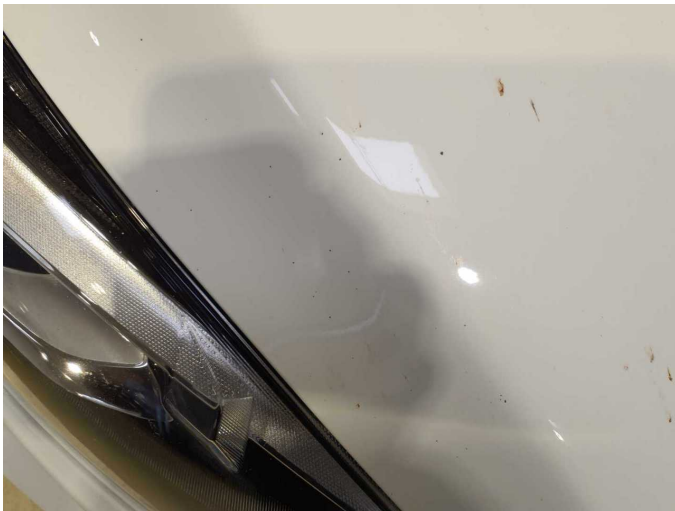
Damage 5: Bonnet: Bonnet - Stone chips - Paint
