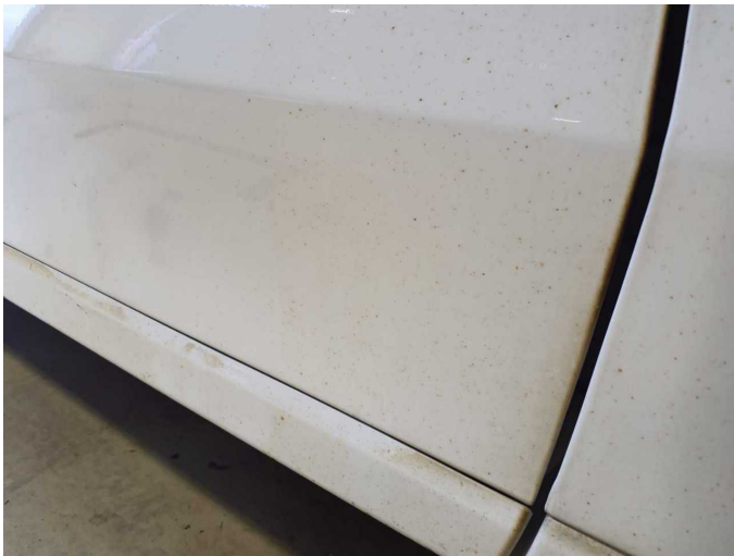
Damage 3: Body: Body (Flugrost) - Soiled - Clean
