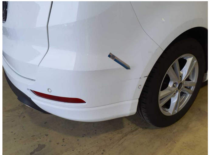
Damage 4: Rear bumper: Rear bumper - Scratch(es) - Paint
