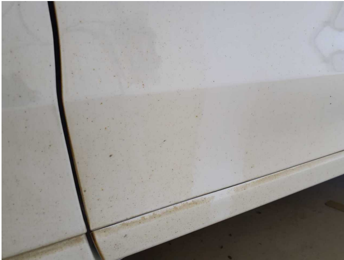
Damage 3: Body: Body (Flugrost) - Soiled - Clean
