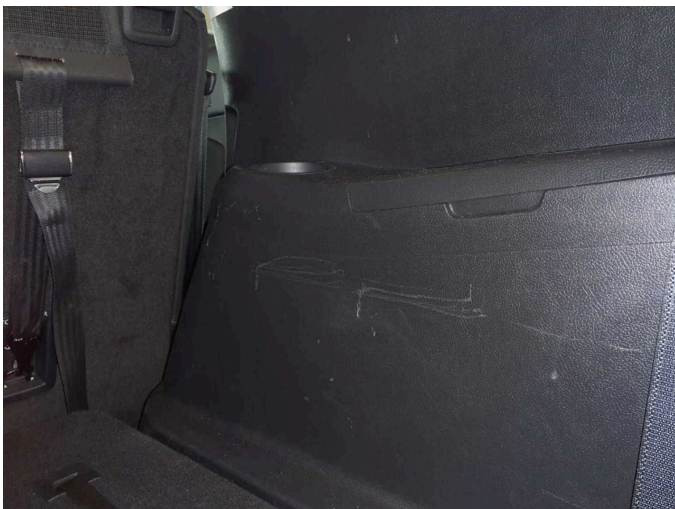
Damage 3: Side panel - rear right side: Interior trim - Scratch(es) - Loss in value
