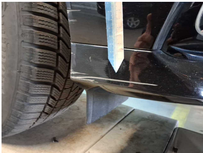
Damage 3: Front bumper: Spoiler - Scratched - Paint
