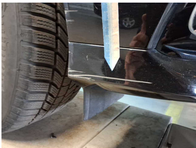
Damage 4: Front bumper: Front bumper - Scratched - Paint
