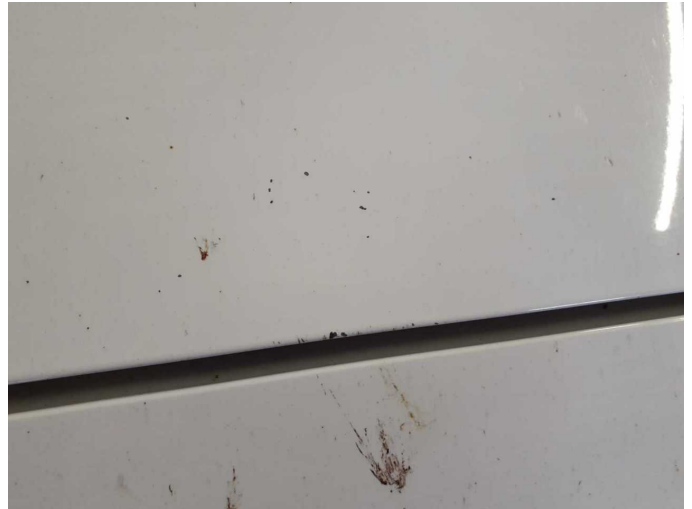
Damage 5: Bonnet: Bonnet - Stone chips - Paint
