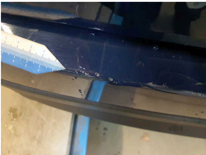
Damage 10: Rear bumper: Rear bumper - Scratched - Paint
