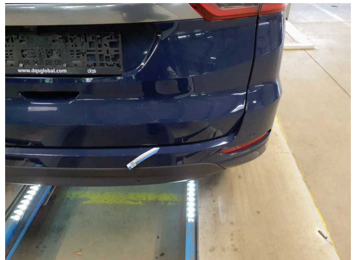
Damage 10: Rear bumper: Rear bumper - Scratched - Paint
