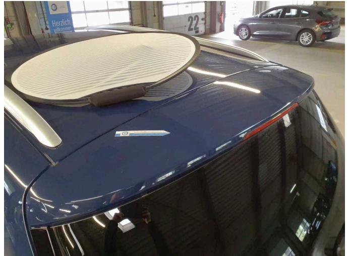
Damage 11: Boot lid / rear door: Rear spoiler - Deformed - Repair and paint
