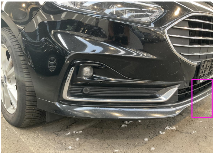
10. Bumper / Front Bodywork / Breakage / Crack -
