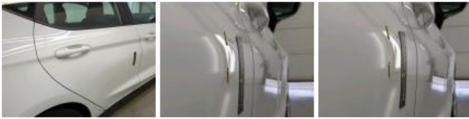
Wing RR, Scratch(es), Repair and paint (complete)
