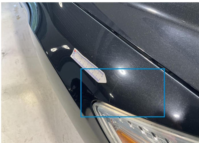
7. Fender / Front Right Paint / Scratch / Scuff -
