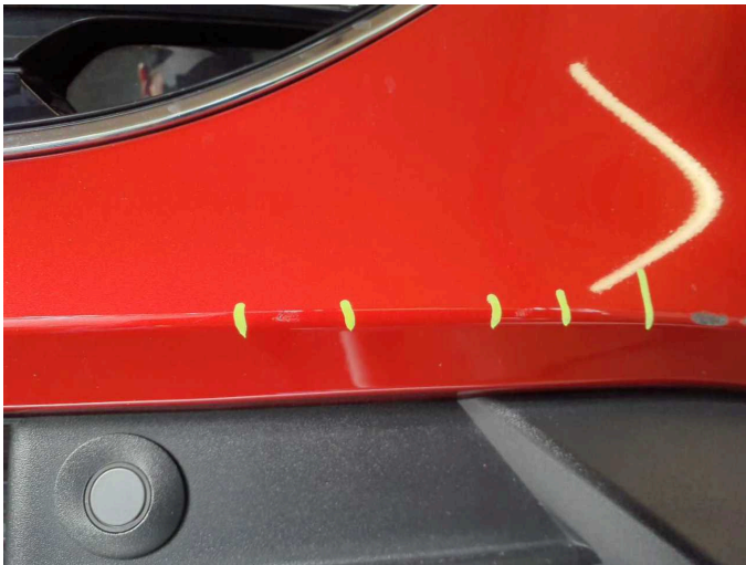
Damage 5: Front bumper: Front bumper - Scratch(es) - Paint
