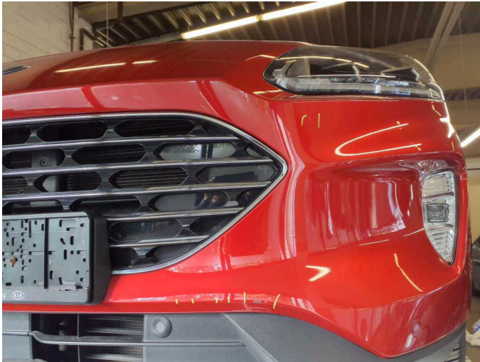
Damage 5: Front bumper: Front bumper - Scratch(es) - Paint
