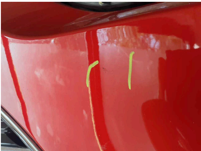
Damage 5: Front bumper: Front bumper - Scratch(es) - Paint
