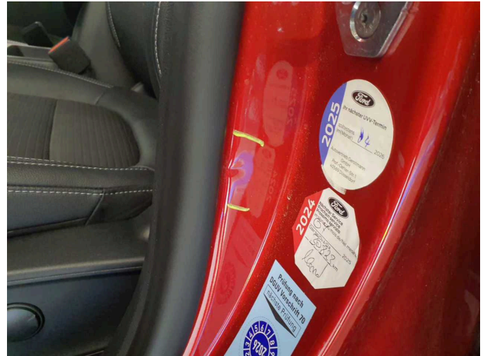
Damage 1: Body: B-pillar - left side - dent(s) - Smart repair
