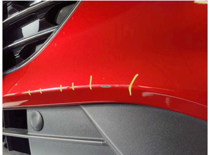
Damage 5: Front bumper: Front bumper - Scratch(es) - Paint
