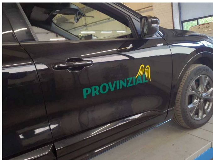
Damage 4: Body: Body - Glued / labelled - De-glue / neutralise
