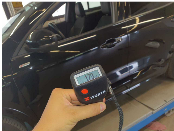
Repainting 1: Mudguard - left side, Bonnet, Door - front left side
