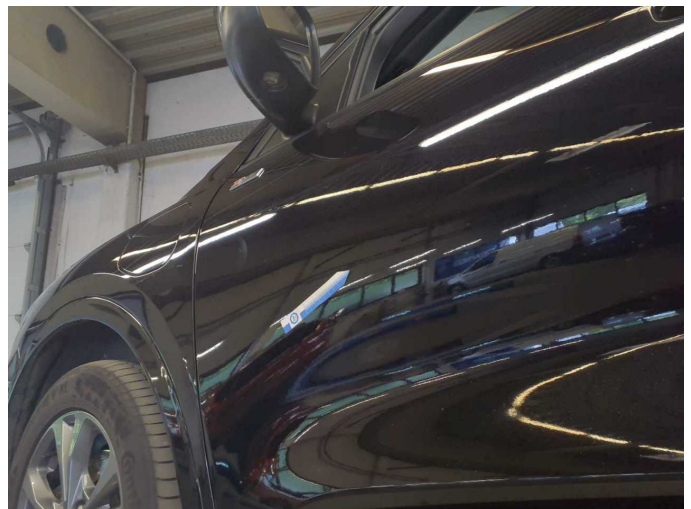
Damage 3: Door - front left side: Door (Lackpickel) - dent(s) - Smart repair
