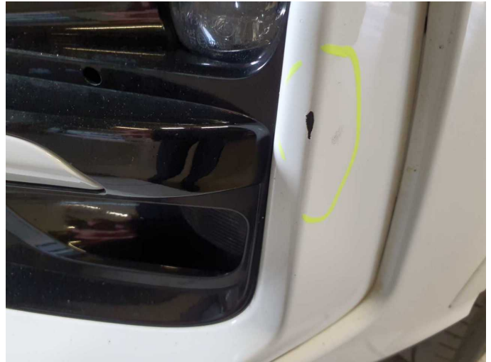
Damage 12: Front bumper: Cover bumper - front (Links) - Scratched - Paint
