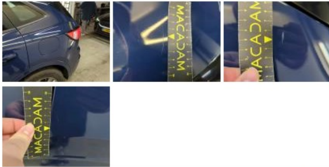
Door RL, Scratch(es), Repair and paint (complete)
