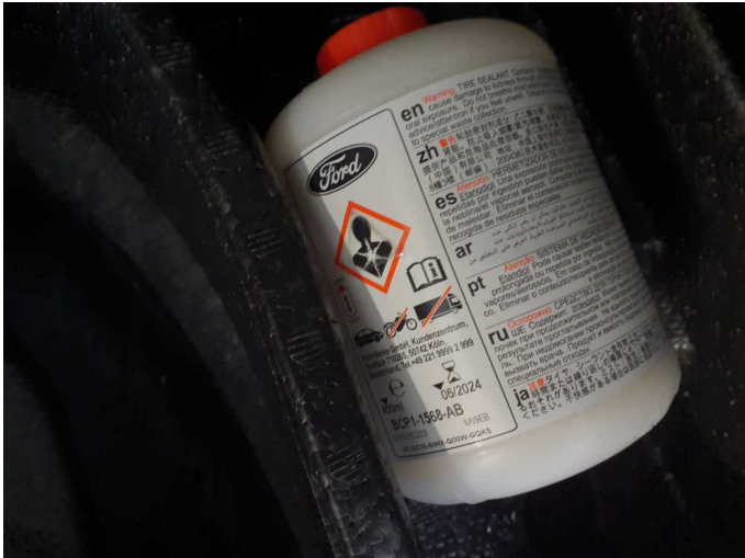
Damage 1: Equipment: Tirefit filler - Expired - Replace
