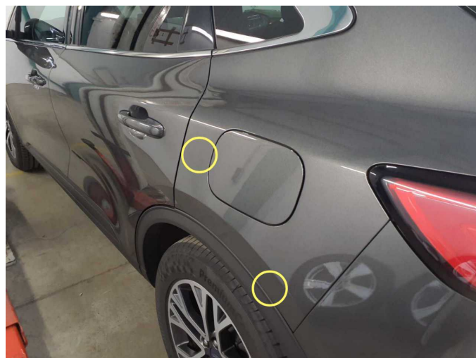
Damage 3: Side panel - rear left side: Side panel (2x) - dent(s) - Smooth repair work
