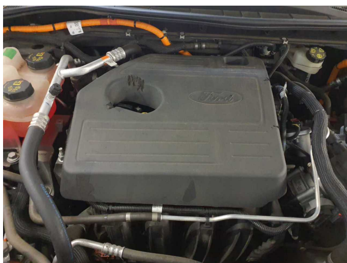
Damage 4: Engine: Engine cover - Damage caused by marten / rodent - Replace
