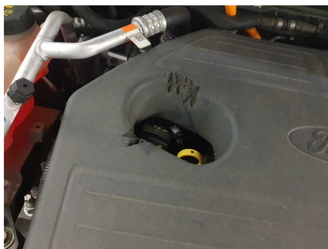
Damage 4: Engine: Engine cover - Damage caused by marten / rodent - Replace
