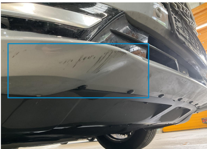
2. Bumper / Front Paint / Scratch / Scuff -
