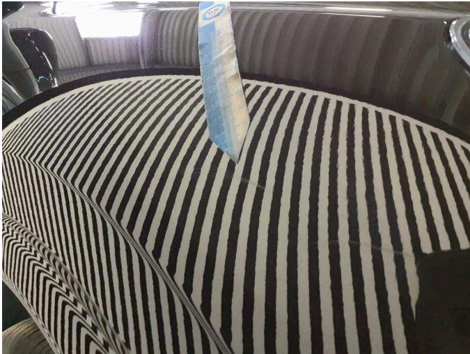
Damage 4: Mudguard - right side: Mudguard - right side - Scratched - Smart repair
