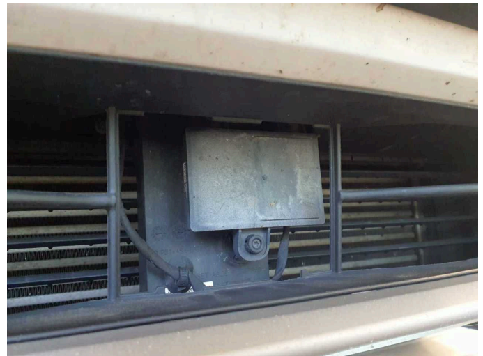
Damage 1: Front bumper: Cap (Grill) - Missing - Replace
