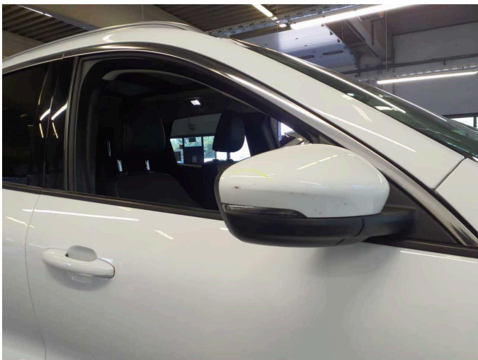
Damage 2: Wing mirror - right side: Cap - Scratch(es) - Smart repair
