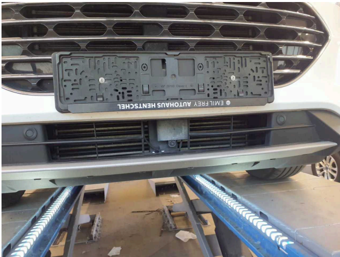
Damage 1: Front bumper: Cap (Grill) - Missing - Replace
