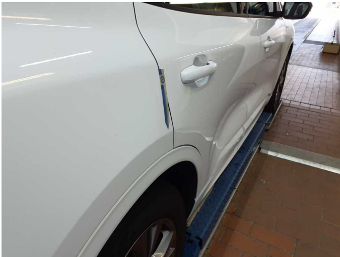
Damage 1: Side panel - rear right side: Side panel - dent(s) - Smart repair
