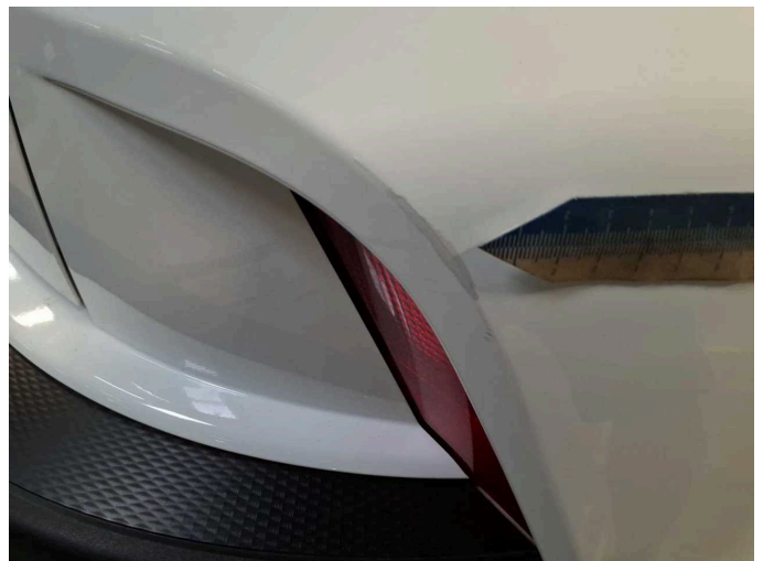
Damage 6: Rear bumper: Bumper - rear right side - Scratch(es) - Paint
