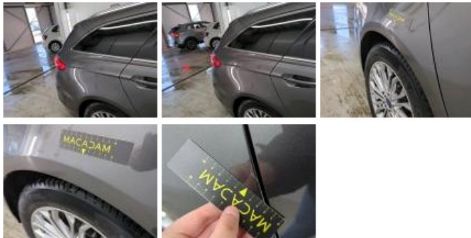
Door RR, Dent(s), Repair and paint (complete)
