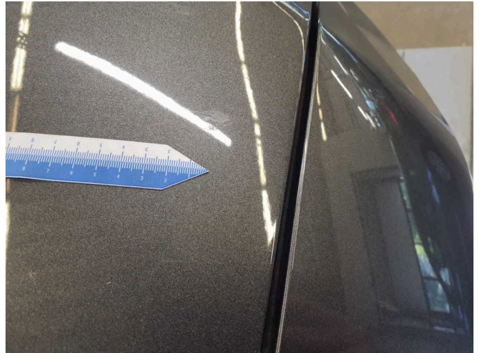
Damage 2: Bonnet: Bonnet (Knick) - Deformed - Smart repair
