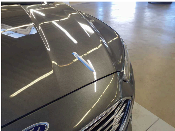
Damage 2: Bonnet: Bonnet (Knick) - Deformed - Smart repair
