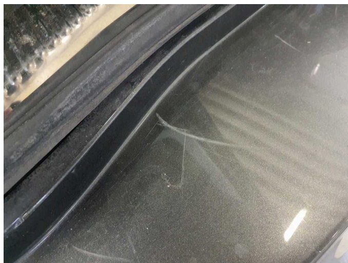
Damage 7: Rear bumper: Rear bumper - Scratch(es) - Paint
