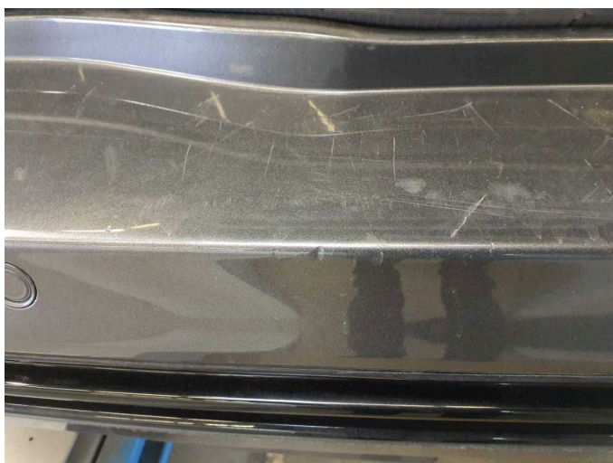
Damage 7: Rear bumper: Rear bumper - Scratch(es) - Paint
