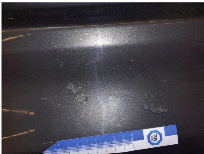
Damage 8: Boot lid / rear door: Trim - standard - lower - Damaged - Replace
