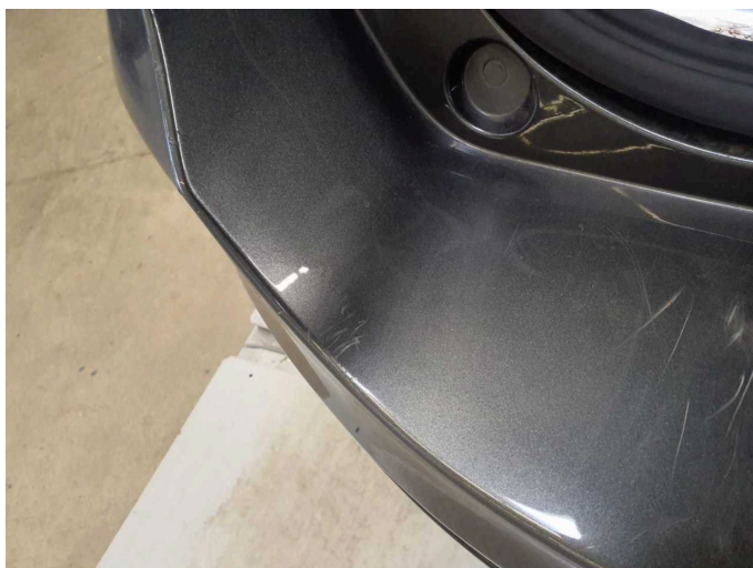
Damage 7: Rear bumper: Rear bumper - Scratch(es) - Paint
