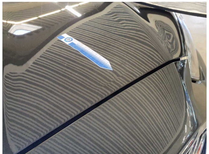
Damage 2: Bonnet: Bonnet (Knick) - Deformed - Smart repair
