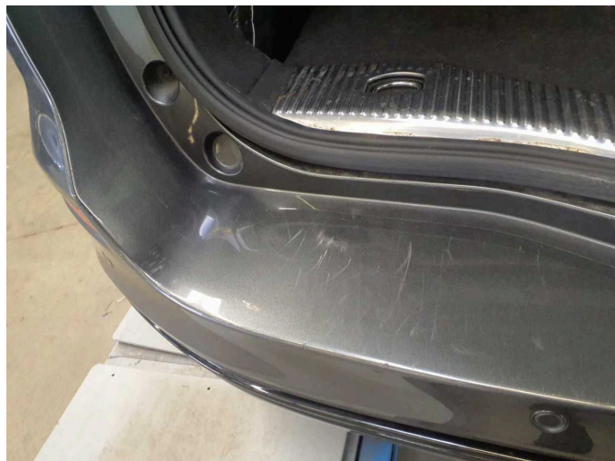
Damage 7: Rear bumper: Rear bumper - Scratch(es) - Paint
