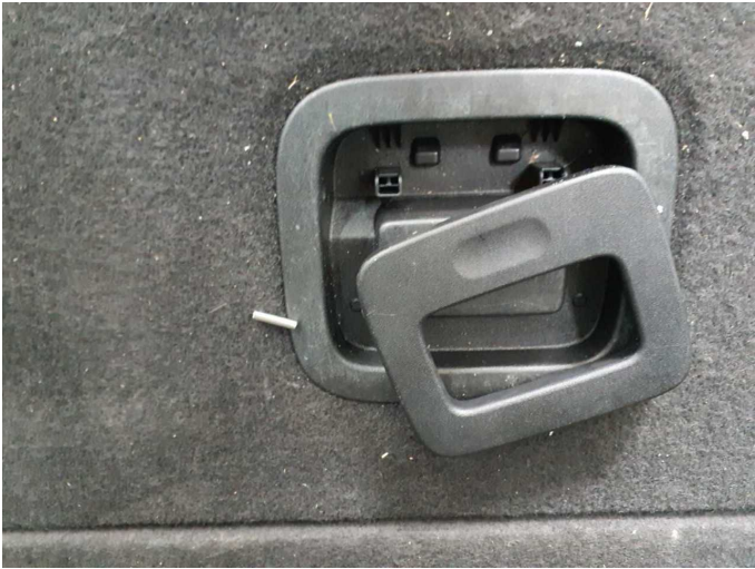
Damage 1: Rear of vehicle: Boot floor (Griff) - Damaged - Replace
