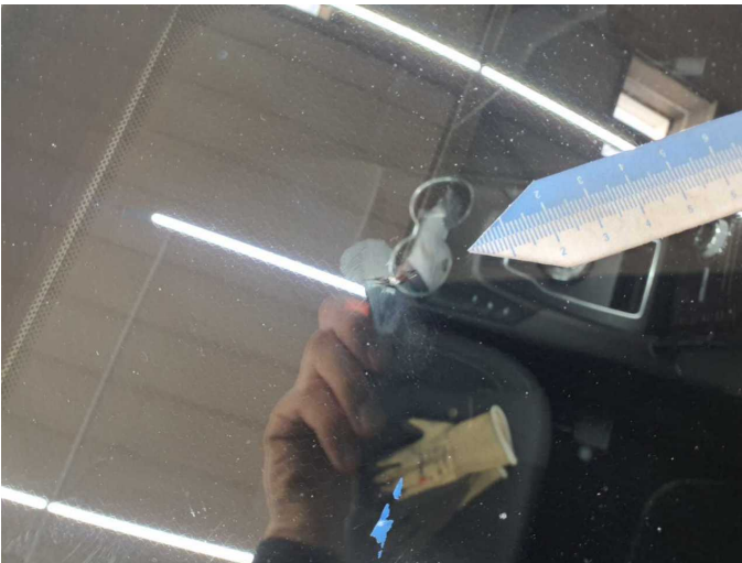
Damage 3: Vehicle glazing: Windscreen - Stone chips - Smart repair
