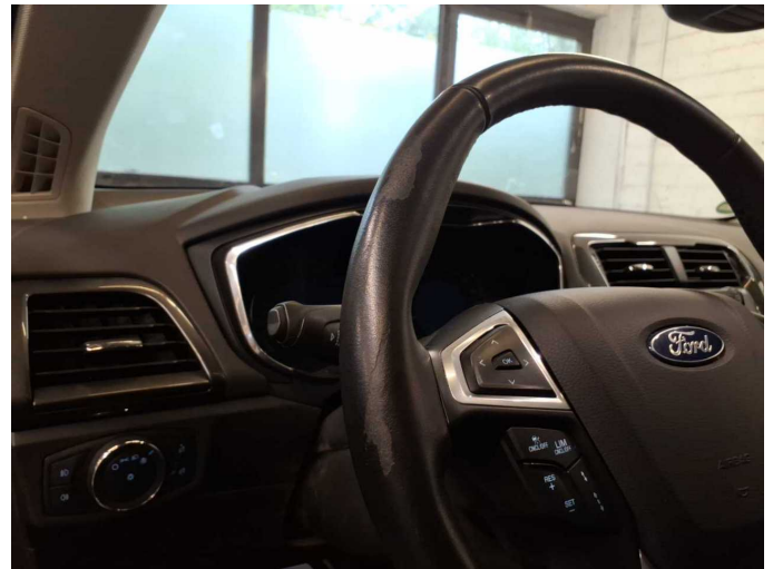
Damage 2: Steering system: Steering wheel - Scratch(es) - Smart repair
