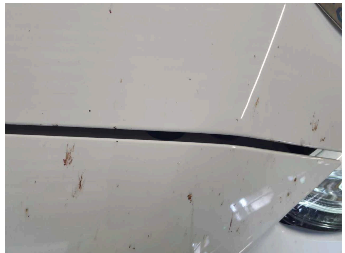
Damage 3: Bonnet: Bonnet - Stone chips - Paint
