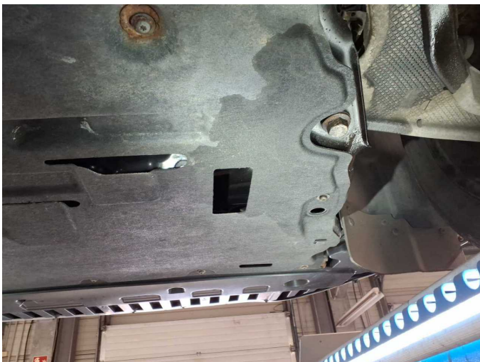
Damage 3: Engine: Engine - Leaking - Perform diagnosis
