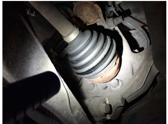
Damage 5: Drive train: Sleeve prop shaft - front right side - Broken / torn - Replace
