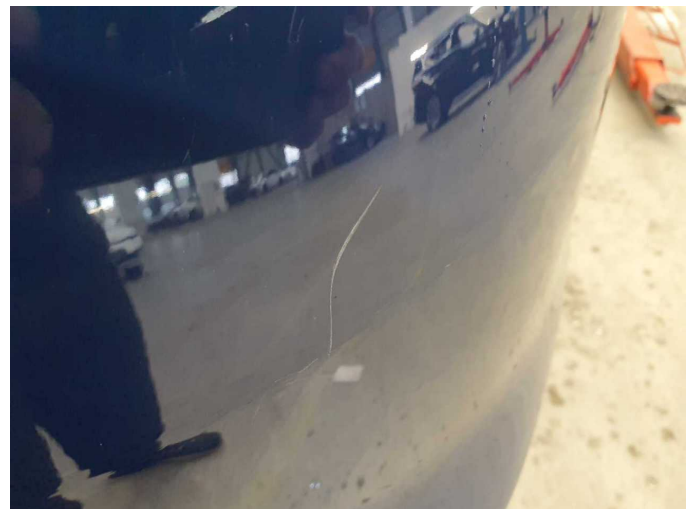
Damage 4: Rear bumper: Rear bumper - Scratch(es) - Paint
