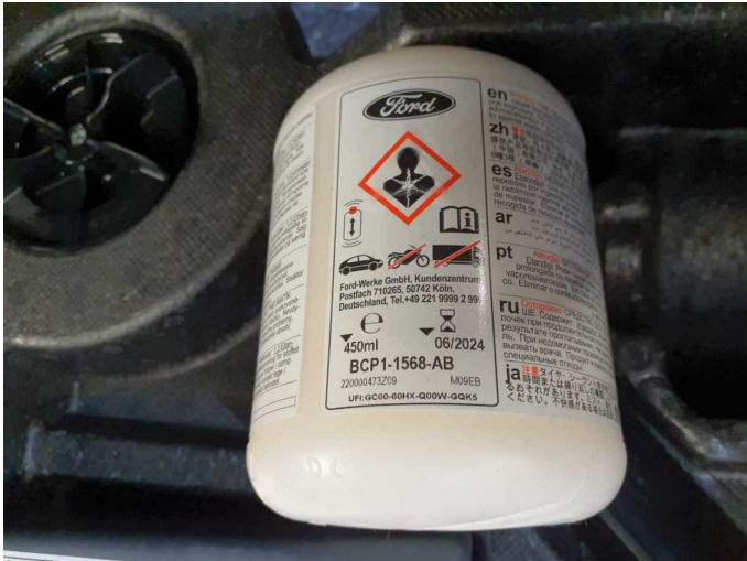
Damage 1: Equipment: Tirefit filler - Expired - Replace
