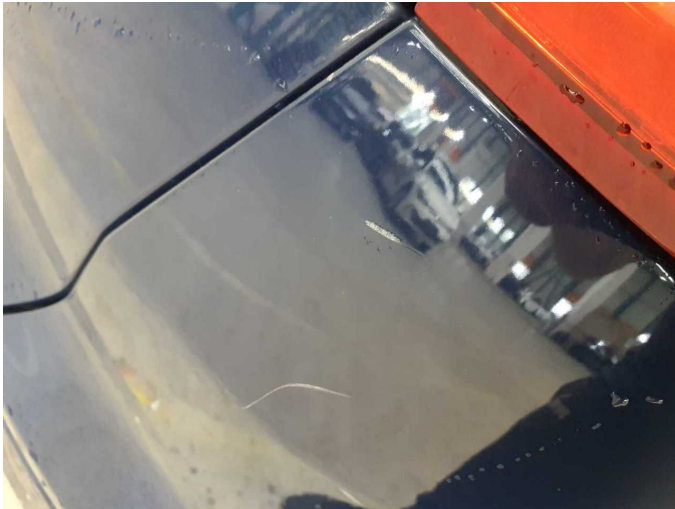
Damage 4: Rear bumper: Rear bumper - Scratch(es) - Paint
