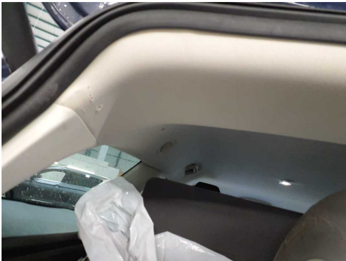
Damage 3: Trim / covers: Roof lining - Broken / torn - Loss in value
