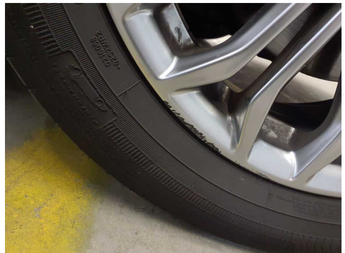
Damage 1: Wheel / tyres: Alloy rim - front right side - Scratch(es) - Smart repair
