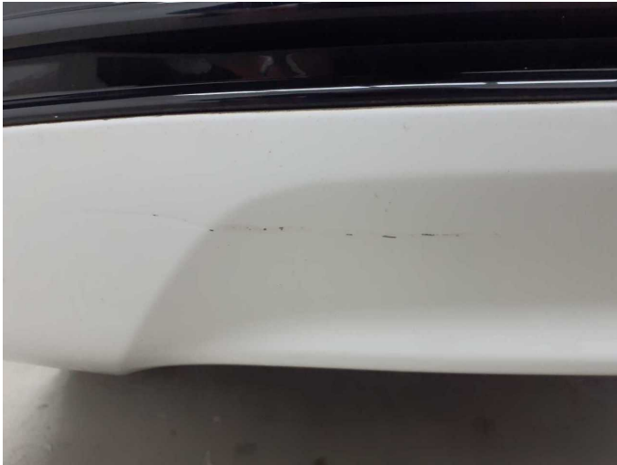
Damage 4: Rear bumper: Rear bumper - Scratch(es) - Paint
