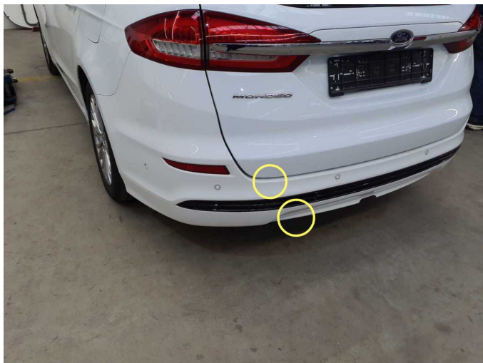
Damage 4: Rear bumper: Rear bumper - Scratch(es) - Paint
