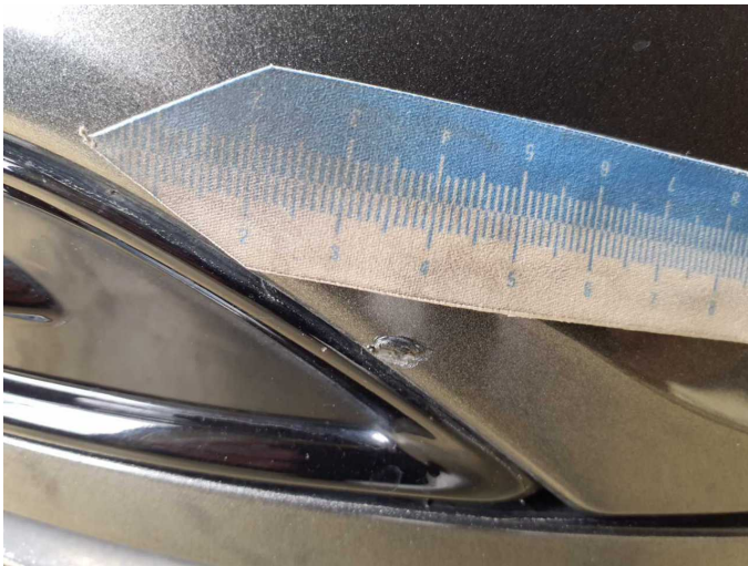
Damage 6: Rear bumper: Rear bumper - Scratch(es) - Paint
