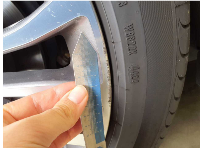
Damage 4: Wheel / tyres: Alloy rim - rear right side - Scratch(es) - Loss in value
