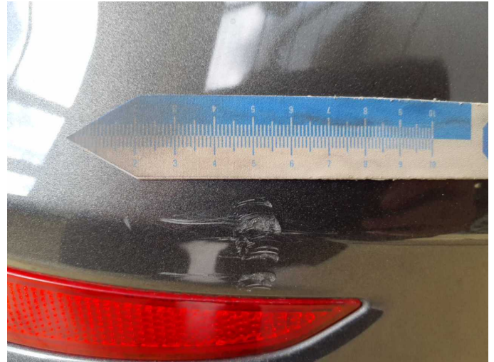
Damage 6: Rear bumper: Rear bumper - Scratch(es) - Paint
