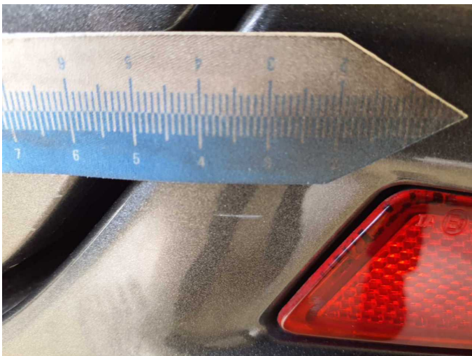
Damage 6: Rear bumper: Rear bumper - Scratch(es) - Paint
