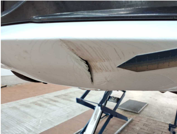
Damage 7: Front bumper: Front bumper - Broken / torn - Replace
