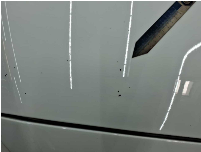
Damage 6: Bonnet: Bonnet - Stone chips - Repair and paint
