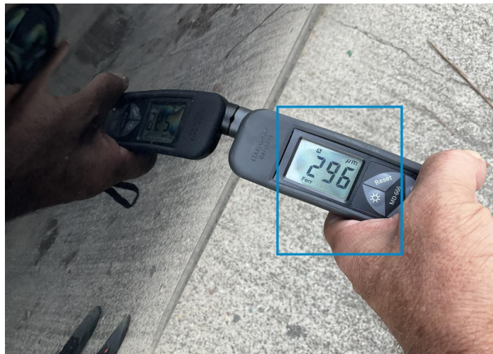
7. Door / Back Right Paint / Poor Previous Repair -
