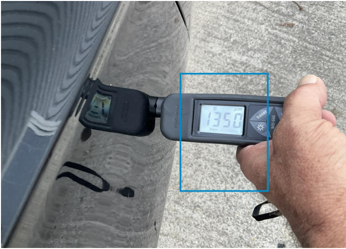
6. Side Panel / Back Right Paint / Poor Previous Repair -
