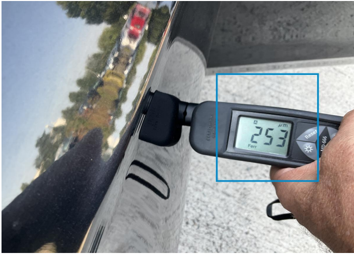
5. Fender / Front Left Paint / Poor Previous Repair -
