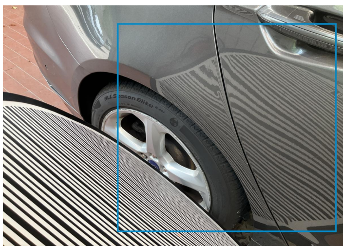
5. Side Panel / Back Right Bodywork / Dent / Dent -
