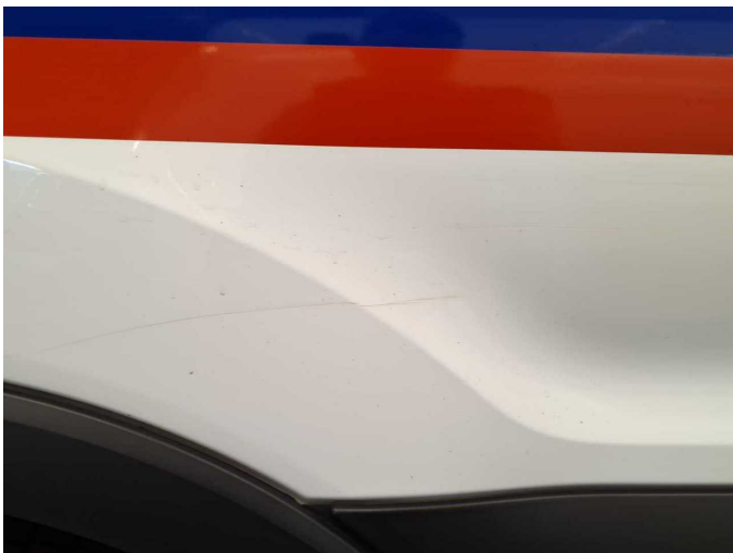
Damage 15: Side panel - rear right side: Side panel (unterhalb) - Dent / paintcoat damage - Repair and paint
