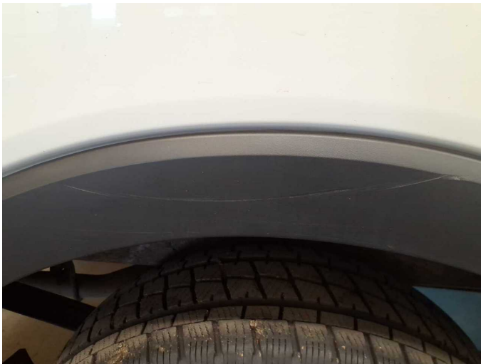
Damage 9: Side panel - rear right side: Wheel arch - Scratch(es) - Replace
