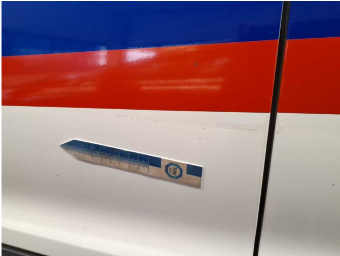
Damage 16: Door - rear left side: Door (Schiebetür) - Dent / paintcoat damage - Repair and paint
