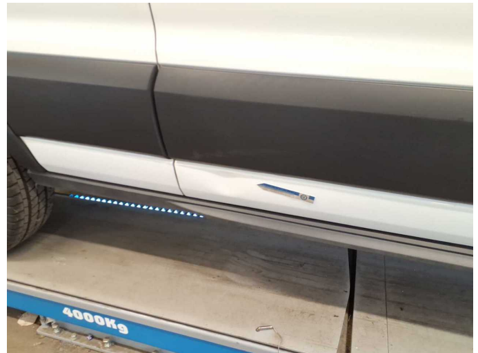
Damage 7: Door - rear right side: Door (Schiebetür) - Deformed - Smart repair
