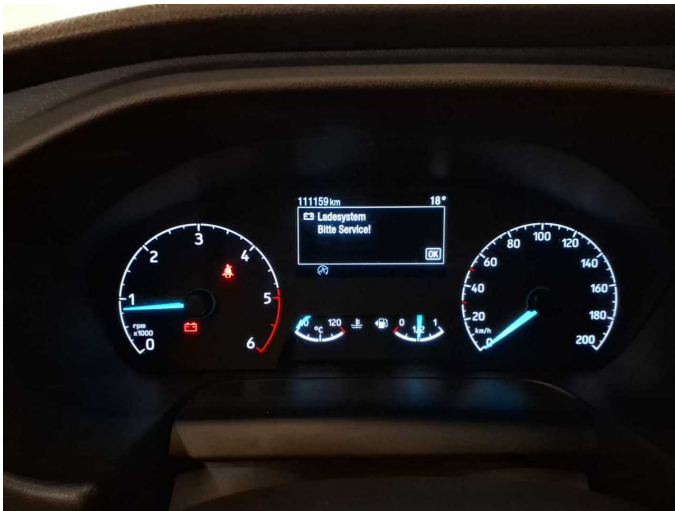
Damage 6: Instrument panel: Indicator light - on - Perform diagnosis
