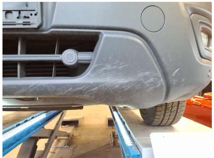
Damage 11: Front bumper: Front bumper (unpainted) - Scratch(es) - Replace
