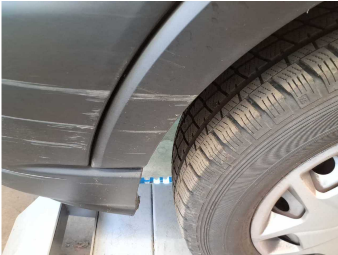
Damage 8: Mudguard - left side: Wheel arch - Scratch(es) - Replace
