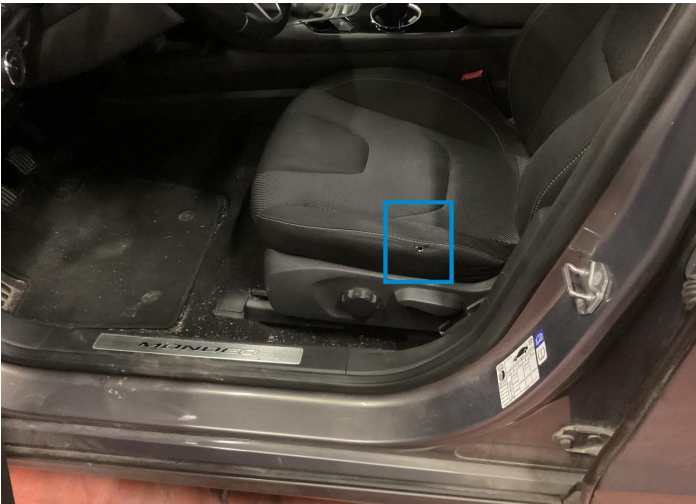
3. Seat Cushion / Front Left Interior / Ripped -
