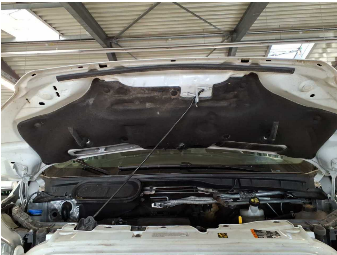
Damage 3: Bonnet: Insulation lining - Broken / torn - Replace
