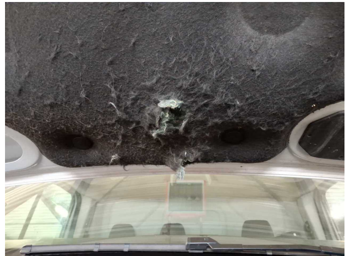
Damage 3: Bonnet: Insulation lining - Broken / torn - Replace
