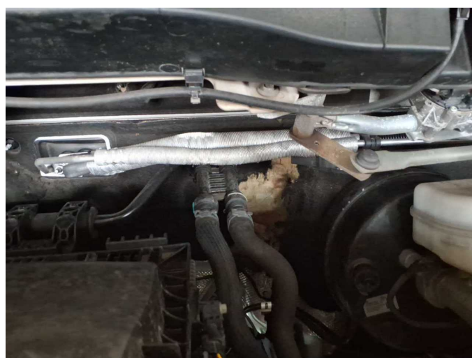
Damage 5: Bonnet: Insulation lining (Spritzwand) - Broken / torn - Replace
