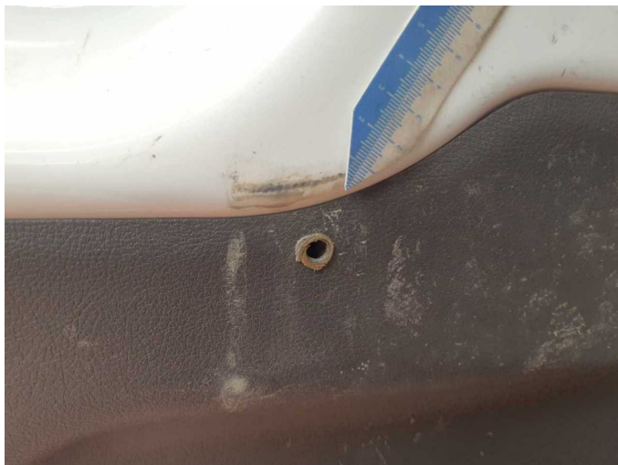
Damage 5: Boot lid / rear door: Trim - standard - lower - Holes - Replace
