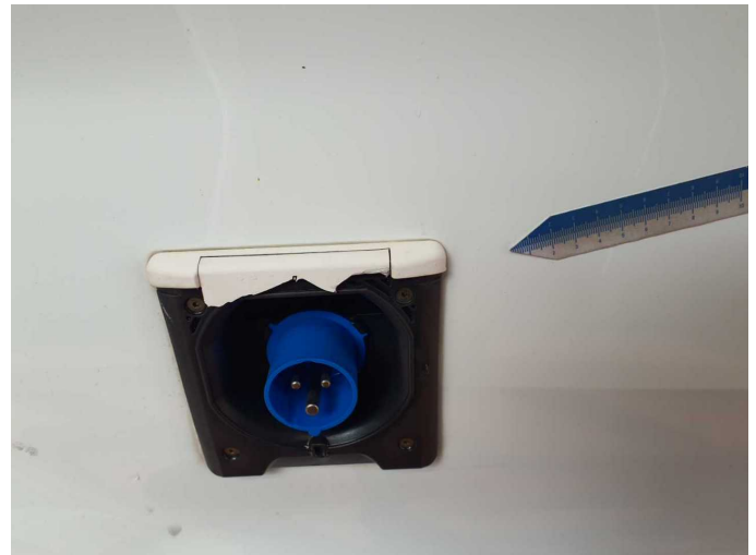
Damage 2: Electrical system: Power socket (Deckel) - Damaged - Replace
