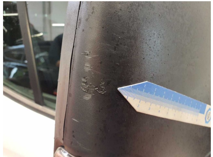
Damage 1: Wing mirror - right side: Cap - Scratch(es) - Replace
