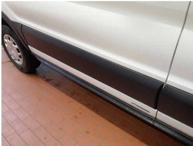
Damage 7: Sliding door, right: Sliding door with glass panel - Dent / paintcoat damage - Smart repair
