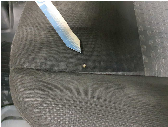
Damage 6: Seat - front: Seat cover - left side - Burn hole (cigarettes) - Loss in value
