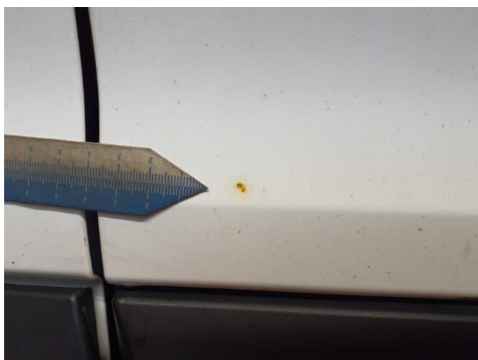
Damage 3: Fuel system: Tank cap (Rost) - Paint defect - Smart repair
