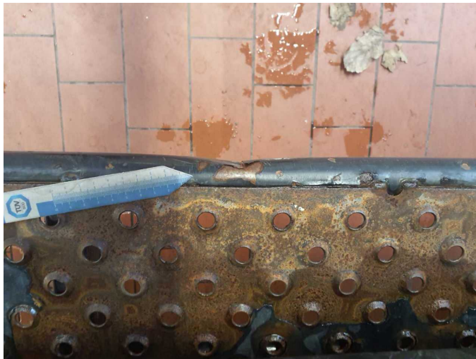
Damage 10: Rear of vehicle: Foot plate - Deformed - Loss in value
