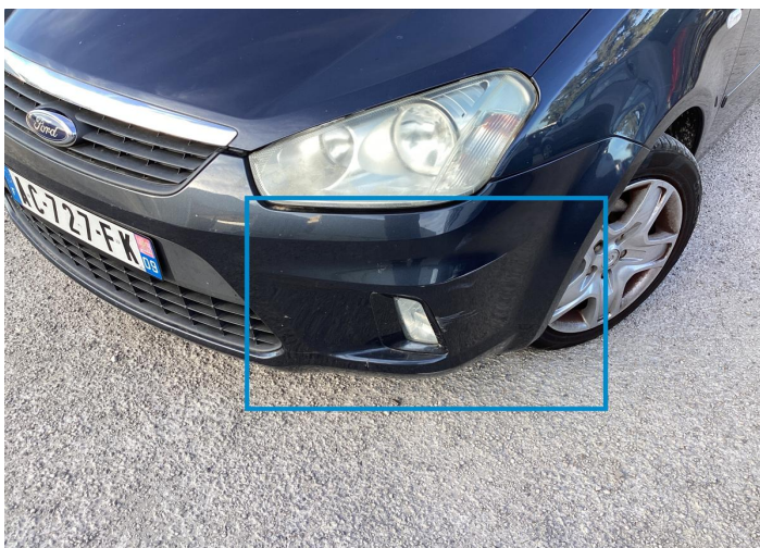
11. Shield / Front Paint / Scratch / Line -
