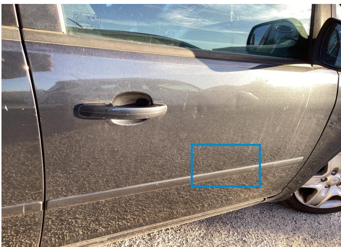
30. Door / Front Right Bodywork / Dent / Deformation -
