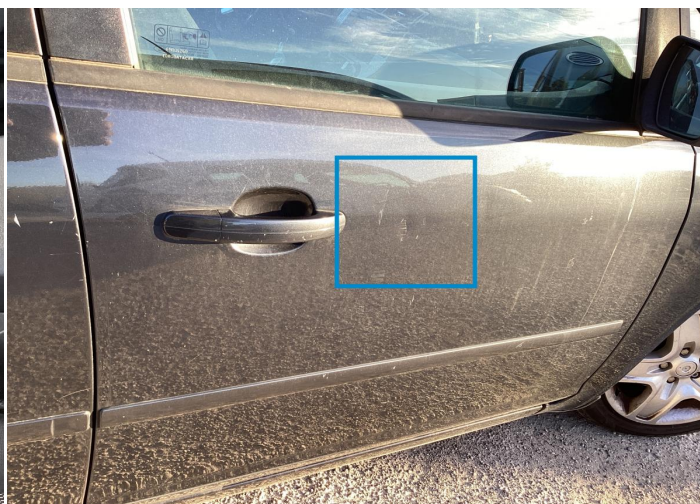
24. Door / Front Right Bodywork / Dent / Deformation -
