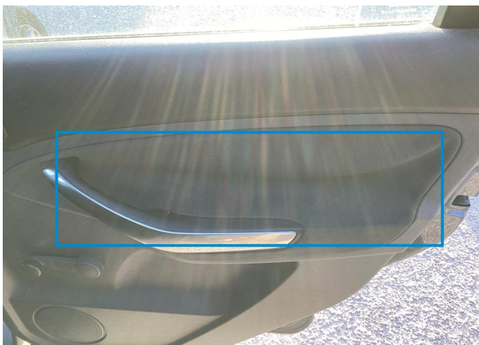
7. Panel Filling / Back Right Interior / Loose -
