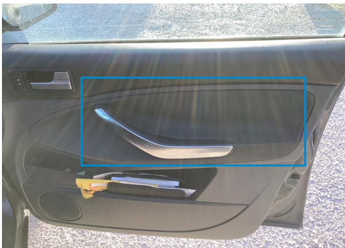
9. Panel Filling / Front Right Interior / Loose -
