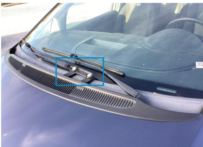
27. Windshield Wiper Blade / Front Right Missing Part -
