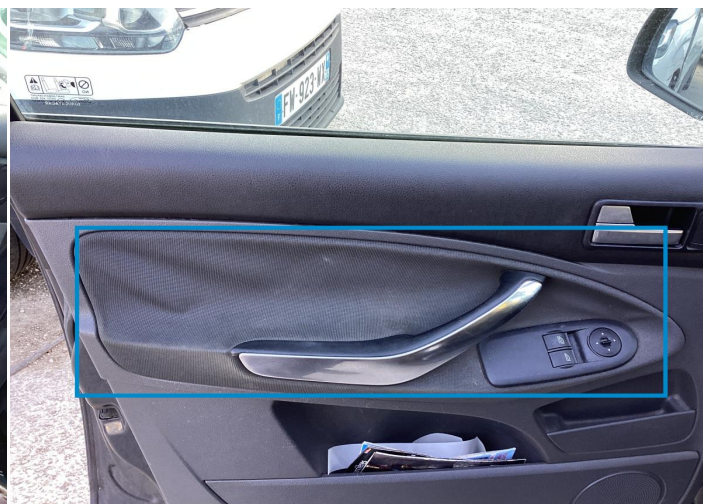
6. Panel Filling / Front Left Interior / Loose -
