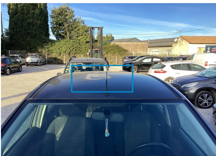
26. Roof Paint / Poor Previous Repair -
