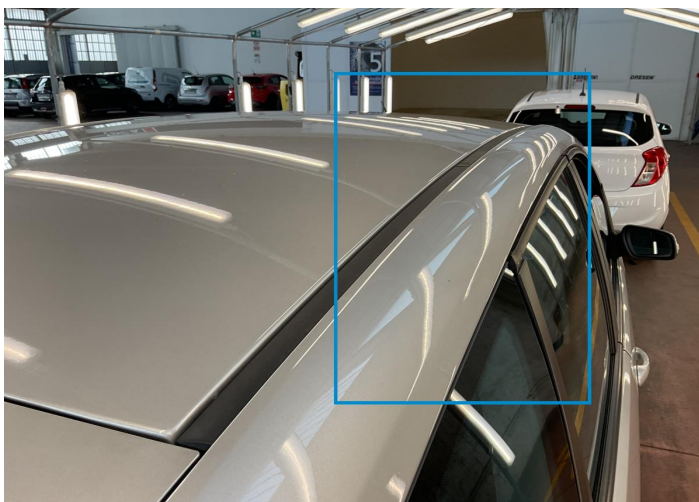
29. Pillar / Front Right Bodywork / Dent / Hail Area -
