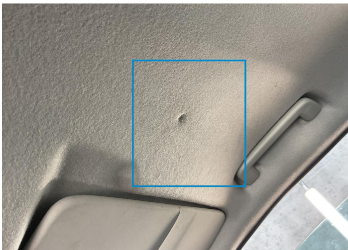
3. Roof Upholstery Interior / Broken -
