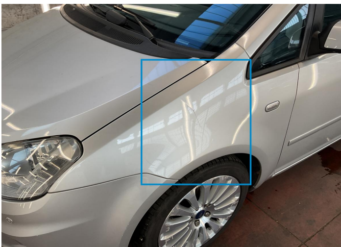
20. Fender / Front Left Bodywork / Dent -
