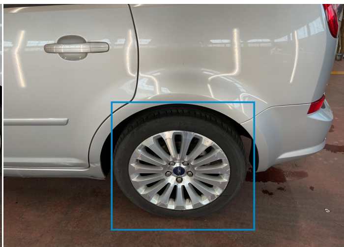
26. Rim / Back Left Out of Bodywork / Scratch -
