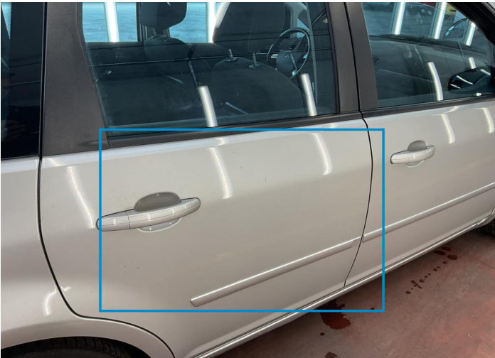
31. Door / Back Right Paint / Scratch / Line -
