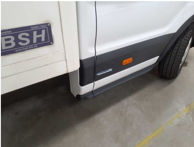
Damage 2: Door - front right side: Brightware - lower - Scratched - Loss in value
