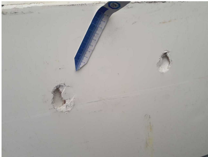
Damage 10: Trim / covers: Cargo area - lining -left side (Teilersatz) - Broken / torn - Repair
