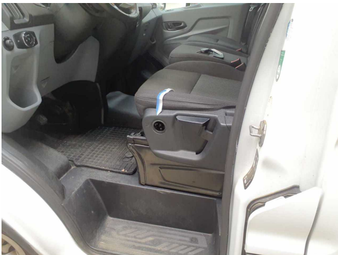
Damage 3: Seat - front: Seat base trim - left side (Blende Sitzverstellung) - Missing - Replace
