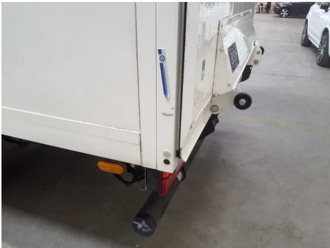
Damage 8: Side panel - rear left side: Side panel (Kofferaufbau inkl. Portalrahmen) - Scratched - Paint
