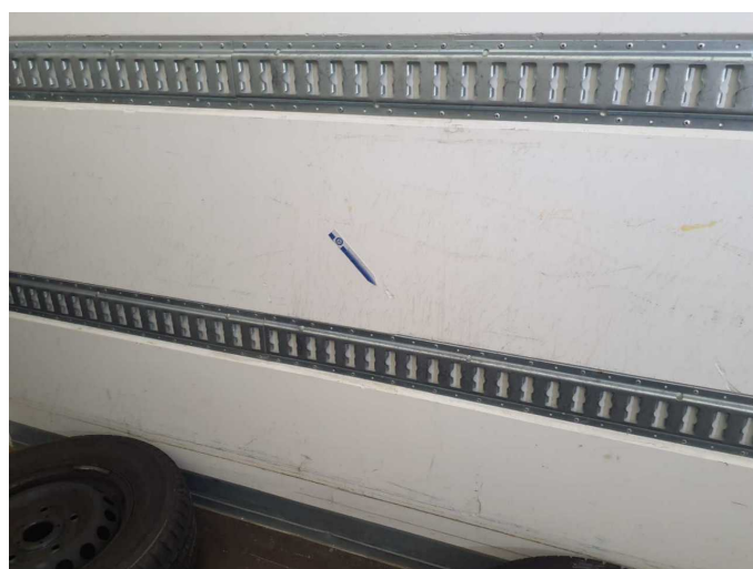
Damage 7: Trim / covers: Cargo area - lining - right side - Scratched - Smart repair
