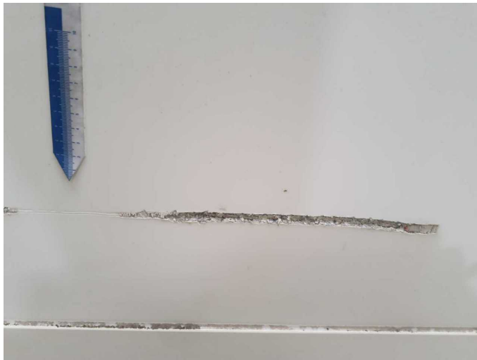
Damage 11: Side panel - rear right side: Side panel (Kofferwand inkl. Portalrahmen hinten) - Scratched - Repair and paint
