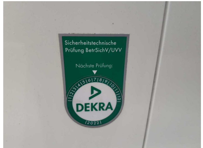
Damage 4: Misc.: Accident prevention regulations tail lift - Expired - Perform
