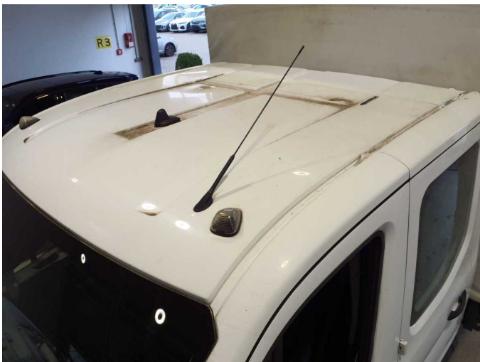
Damage 7: Roof: Roof - Corrosion - Repair and paint
