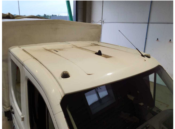
Damage 7: Roof: Roof - Corrosion - Repair and paint
