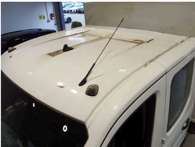
Damage 7: Roof: Roof - Corrosion - Repair and paint
