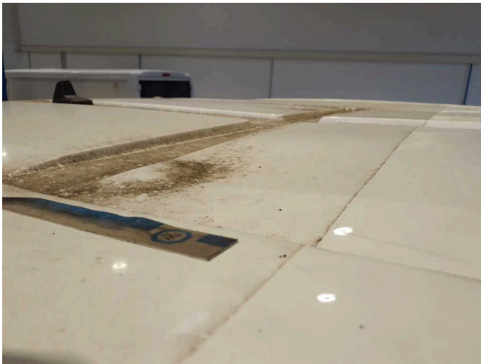
Damage 7: Roof: Roof - Corrosion - Repair and paint
