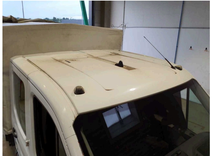
Damage 7: Roof: Roof - Corrosion - Repair and paint
