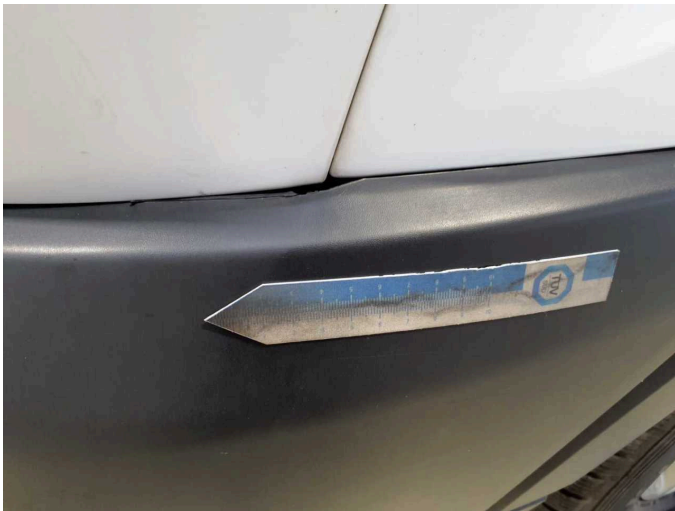
Damage 6: Front bumper: Front bumper (unpainted) - Deformed - Replace
