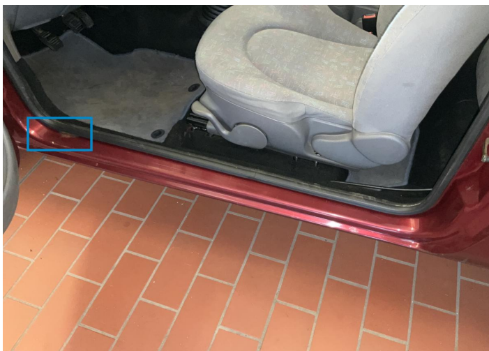
15. Rocker Panel / Center Left Paint / Corrosion -
