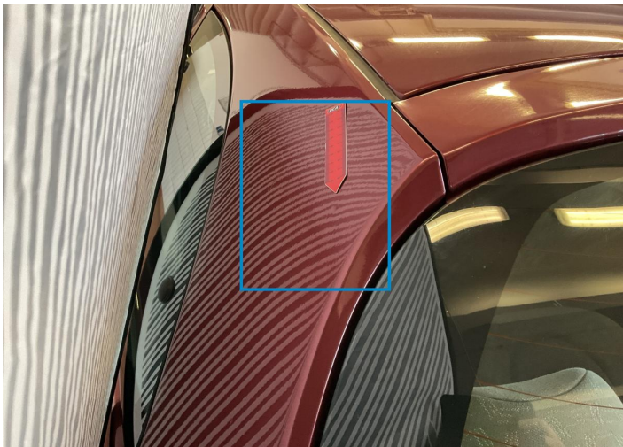
5. Fender / Back Left Bodywork / Dent / Dent -
