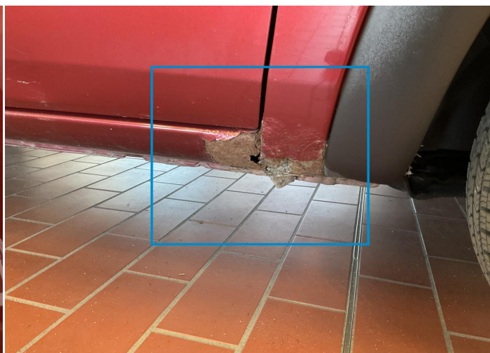
8. Rocker Panel / Center Right Paint / Corrosion -
