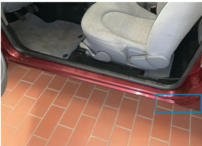
16. Rocker Panel / Center Left Paint / Corrosion -
