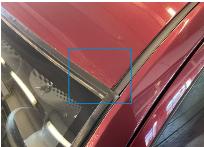
11. Roof Paint / Corrosion -
