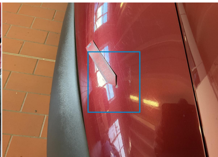
12. Fender / Front Right Paint / Chipping -
